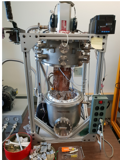
Figure 1.5: The cryostat used for this experiment can reach temperatures down to 50K
