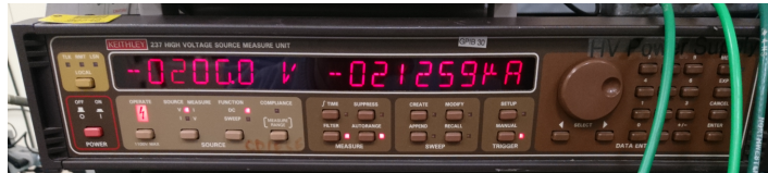
Figure 12: KEITHLEY 237 power supply. It was also used to measure the total current flowed through the detector.
