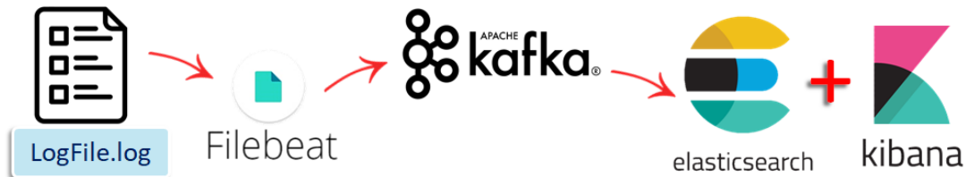
Figure 2: The “chain of software” needed to bring the monitoring data to Elasticsearch from the log file.
