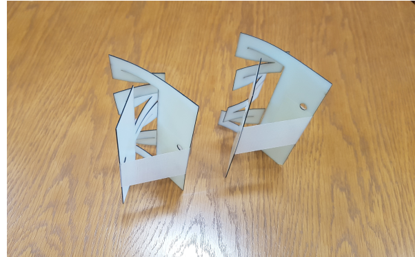
Figure 16: Samples are kept folded overnight to get a first insight of relaxation phenomena.
