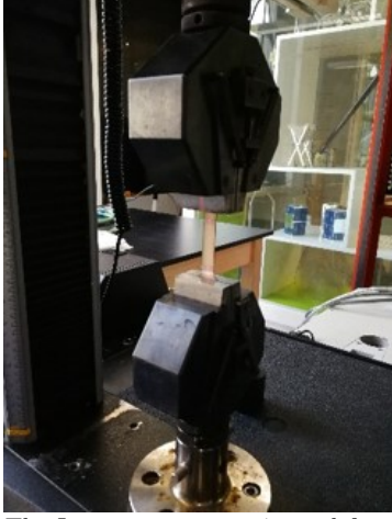
Figure 4: The Instron apparatus is used for tensile tests. The strain is monitored by a laser.
