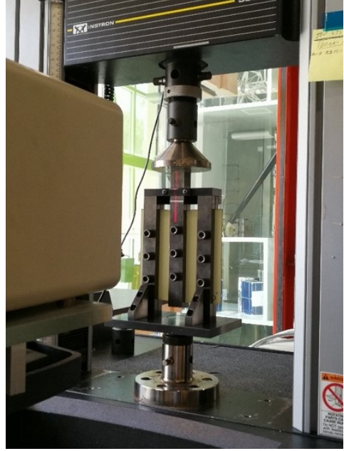
Figure 6: The Instron apparatus is used for shear tests. The displacement is monitored by a laser while the central strip is pushed downwards.
