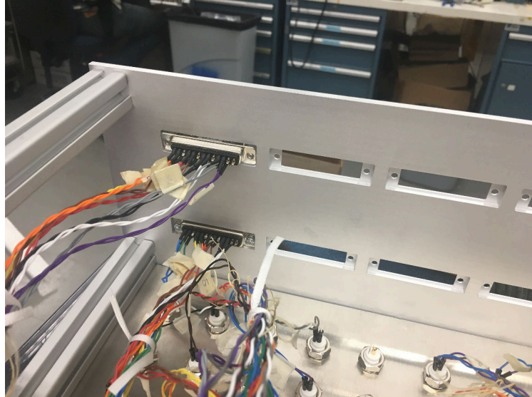
Figure 3.0.5: View on the back of the top plate: this perspective shows the slots extruded in the plate to host the D-sub connectors.
