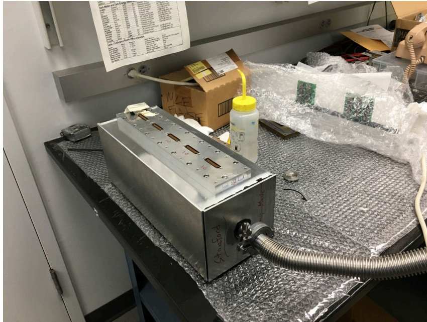
Figure B.0.1: The jig used for the feedthrough leak test; on the top side of the jig there is one of the flanges tested.
