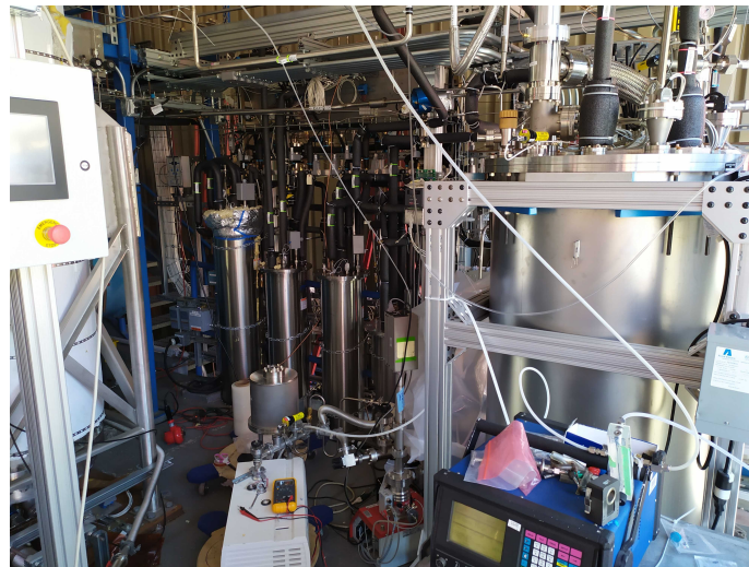
Figure 10. On the left the 4 metals cylinders are the cold Kr traps, on the right the larger cylinder inside the holding structure is the Xe freezer.
