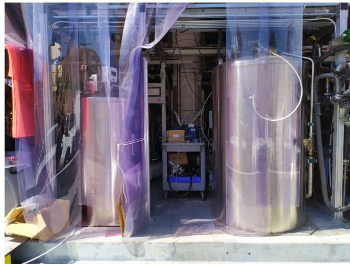
Figure 11. 450L dewar (left) and 1000L dewar (right).
