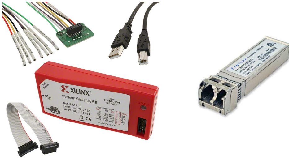
Figure 5.6: On the left: the HW-USB-II-G Xilinx programmer with JTAG connection. On the right: the Finisar FTLX8574D3BCV (50 nm VCSEL 1G/10G Dual-Rate) used as bi-directional communication module between DTC and ROC.
