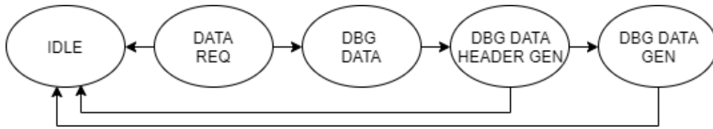
Figure 6.12: State Machine of the Debug Mode in Data Request inside Command Handler
