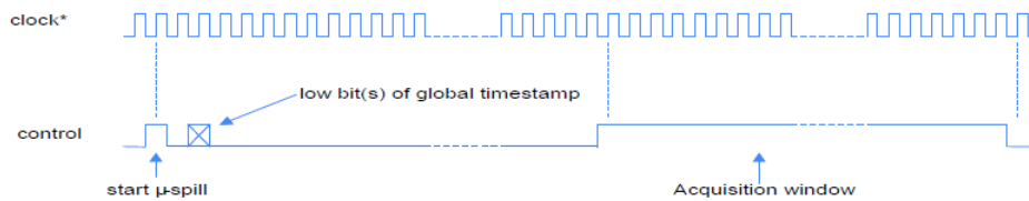
Figure 4.4: A timing diagram for the ROC to digitizer signal transfer. The architecture shows the 200 MHz clock aligned with the \mu spill and the \mu spill ID with the data capture gate. The lowest 4 bits of the \mu spill are transferred on this LVDS line.
