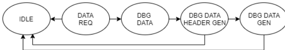
Figure 6.12: State Machine of the Debug Mode in Data Request inside Command Handler
