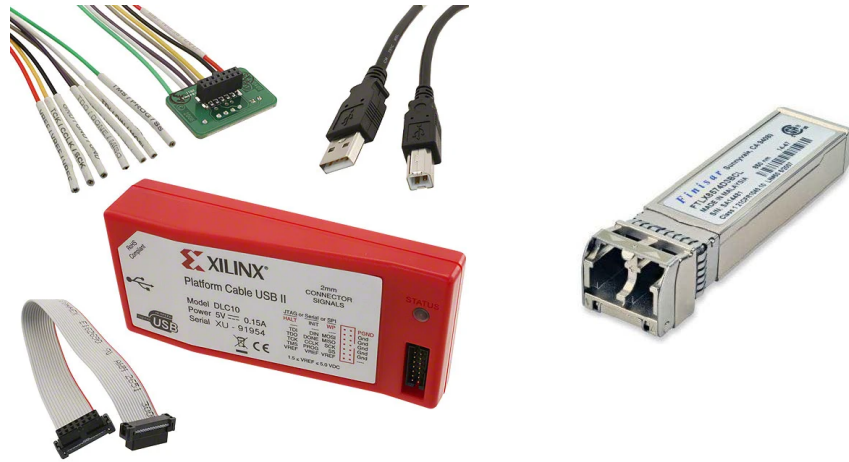
Figure 5.3: On the left: the HW-USB-II-G Xilinx programmer with JTAG connection. On the right: the Finisar FTLX8574D3BCV (50 nm VCSEL 1G/10G Dual-Rate) used as bi-directional communication module between DTC and ROC.
