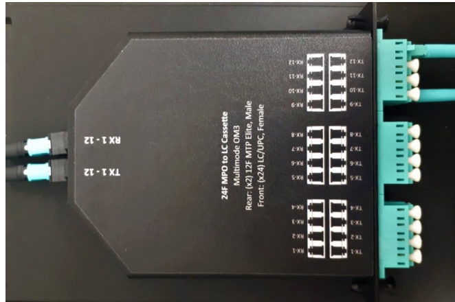
Figure 5.2: Fiber cassette: it is the optical splitter from 12(x2) MTP Male to 24 LC/UPC Female.
