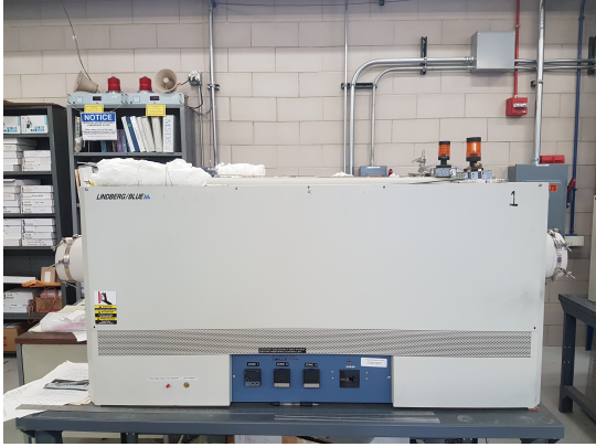
Figure 6: Oven for the thermal treatment, Technical Division, Fermilab
