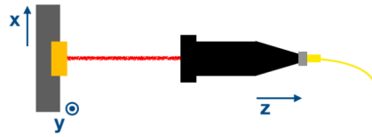
Figure 3.7: Sketch of stage positions. The X and Y axes stages move the device tested, Z stage moves the laser.
