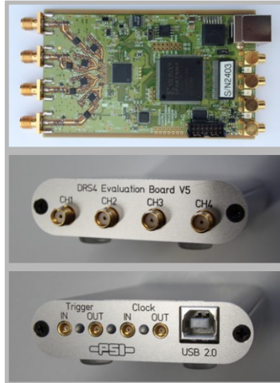
Figure 3.8: The DRS4 board used as 1 GHz 4-channel oscilloscope.
