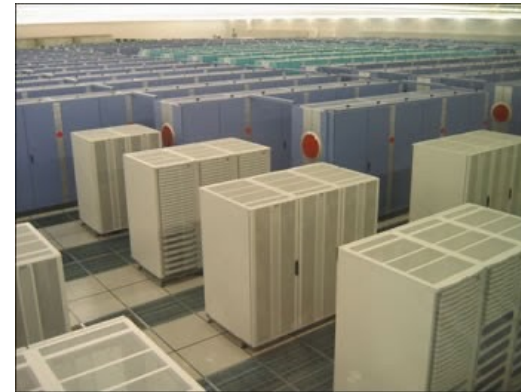
(2002) Earth Simulator: 640 nodes, 35.8 TFLOPS
