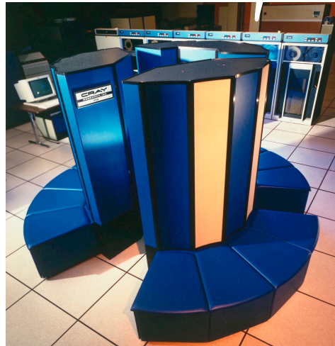
(1985) Cray-2 Supercomputer: 250 MHz cpu, 1.9 GFLOPS
