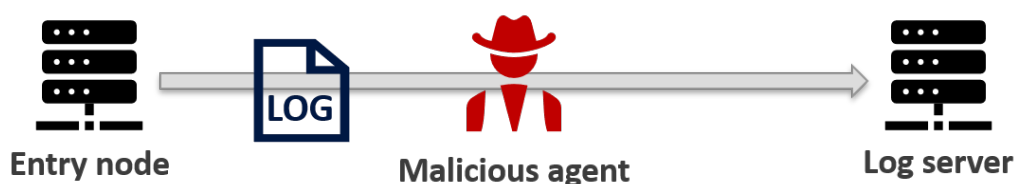
Figure 5: A "man in the middle" in the network between the glidein and the log server can intercept and manipulate the packet if no security mechanism is enforced.
