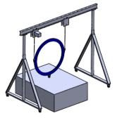
• The wheel can be easily installed when the plane is horizontal and placed on spacers, stands or something similar
