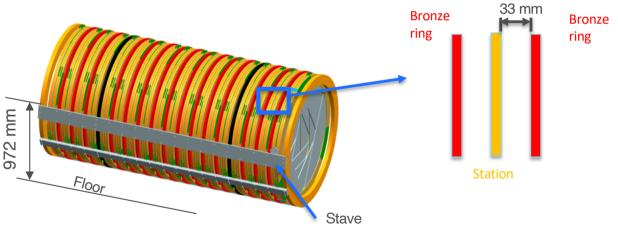
Main geometric constraints of the installation in the frame
