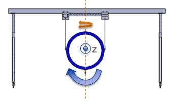
The problem of a lifting system that uses chains are oscillations: the use of two trolleys limits oscillations around vertical axis and z-axis but not around the l-beam axis
