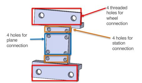
Conceptual design of the flange adapter
