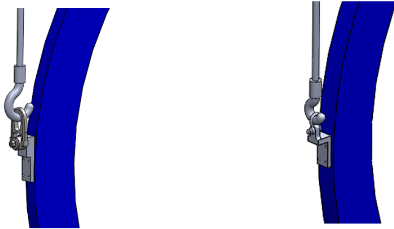
Figure 27: Two conceptual design for the plane lifting brackets: Hoist ring solution (on the left) and Shackle solution (on the right).
