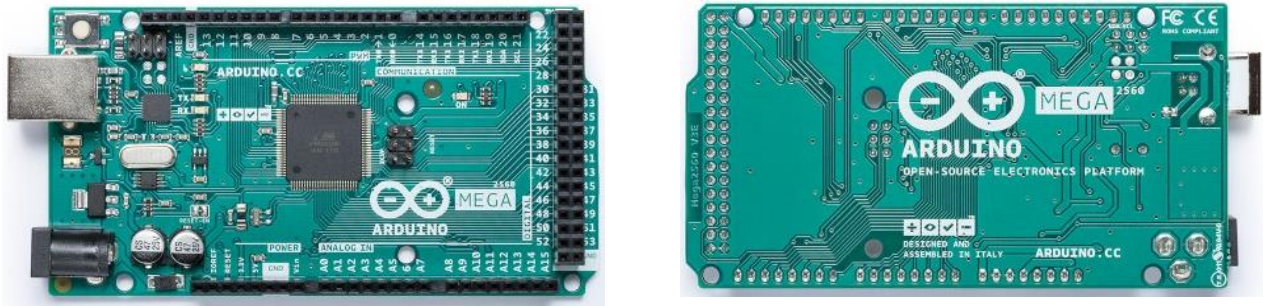
Figure 7: Arduino Mega 2560 board top and bottom view
