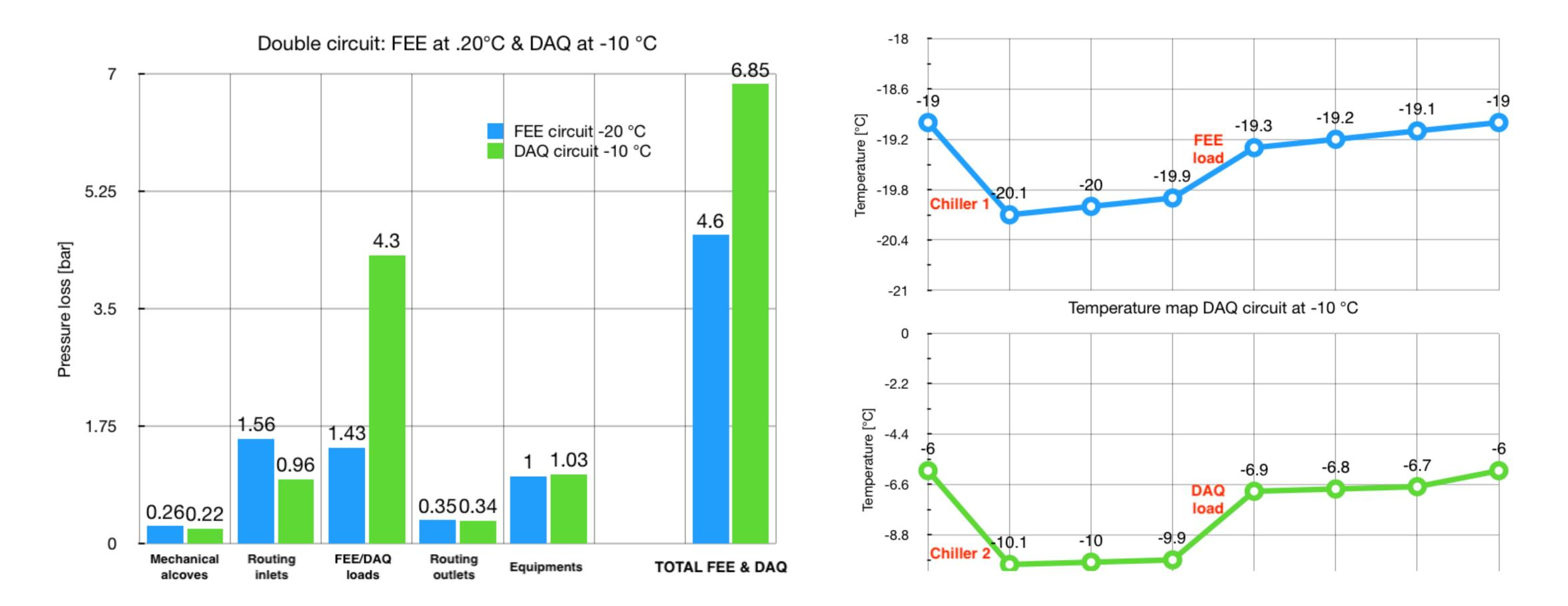
2 Different pumping requirements: 2 kg/s at 7.5 bar for DAQ, and 2.5 kg/s at 5.1 bar for FEE (including safety margins)
