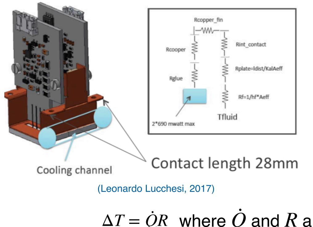
From simulations the temperature difference between fluid and SiPM is around **6.2** °C
