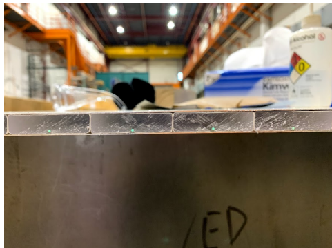
(a) Scintillator before treating it with sandpaper.
