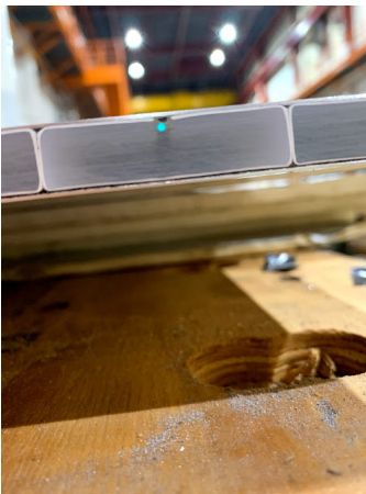
(b) Scintillator after treating it with sandpaper.
