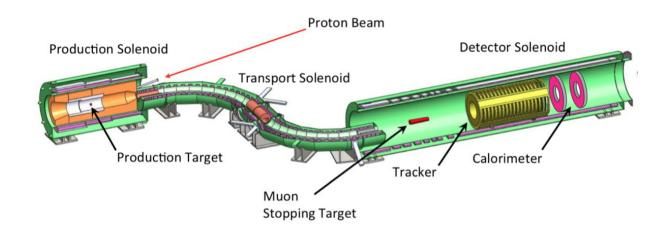
Mu2e has been designed and is currently being constructed at Fermilab to search for the neutrino-less muon conversion to an electron in the field of an aluminum nucleus
