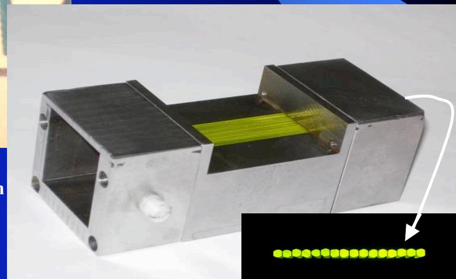
Alpha particles detector (both ends detection)
