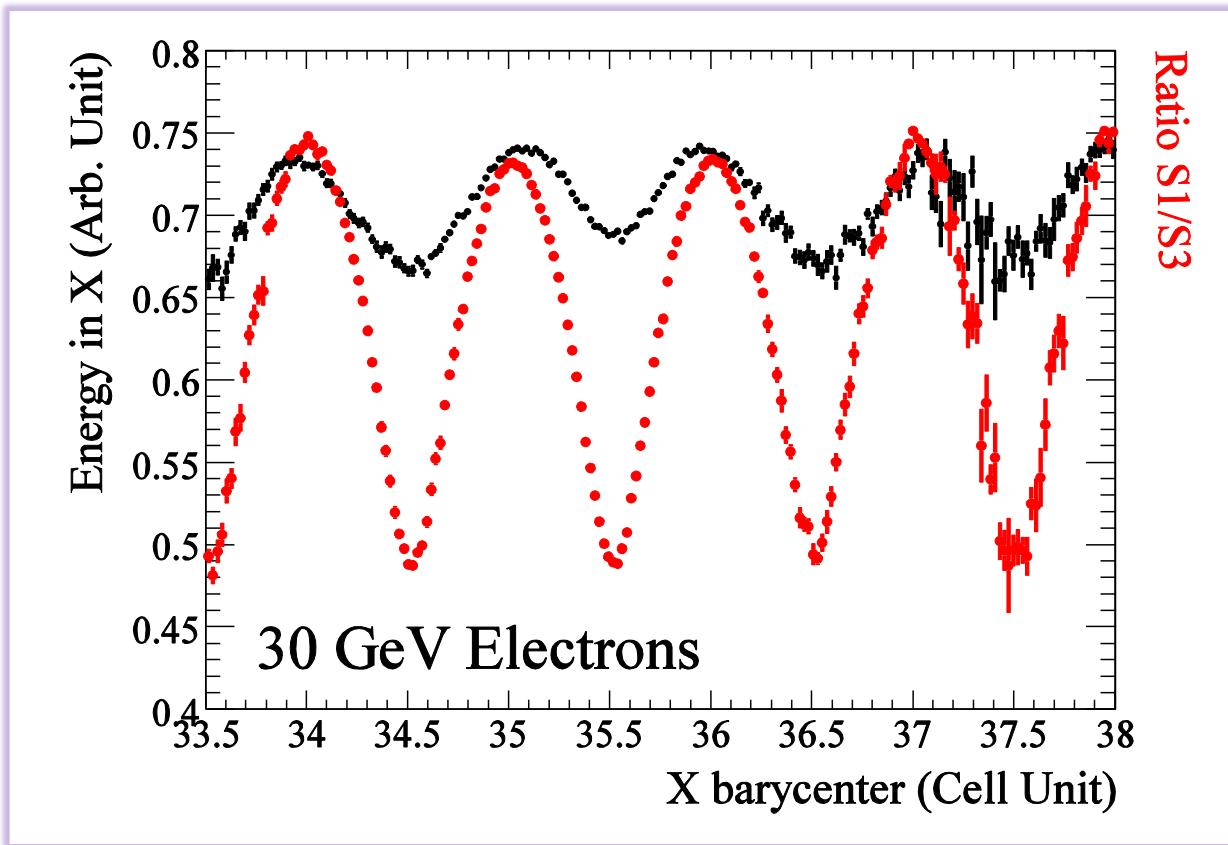
S1/S3 ratio has a better sensitivity to the barycenter than the total energy.
