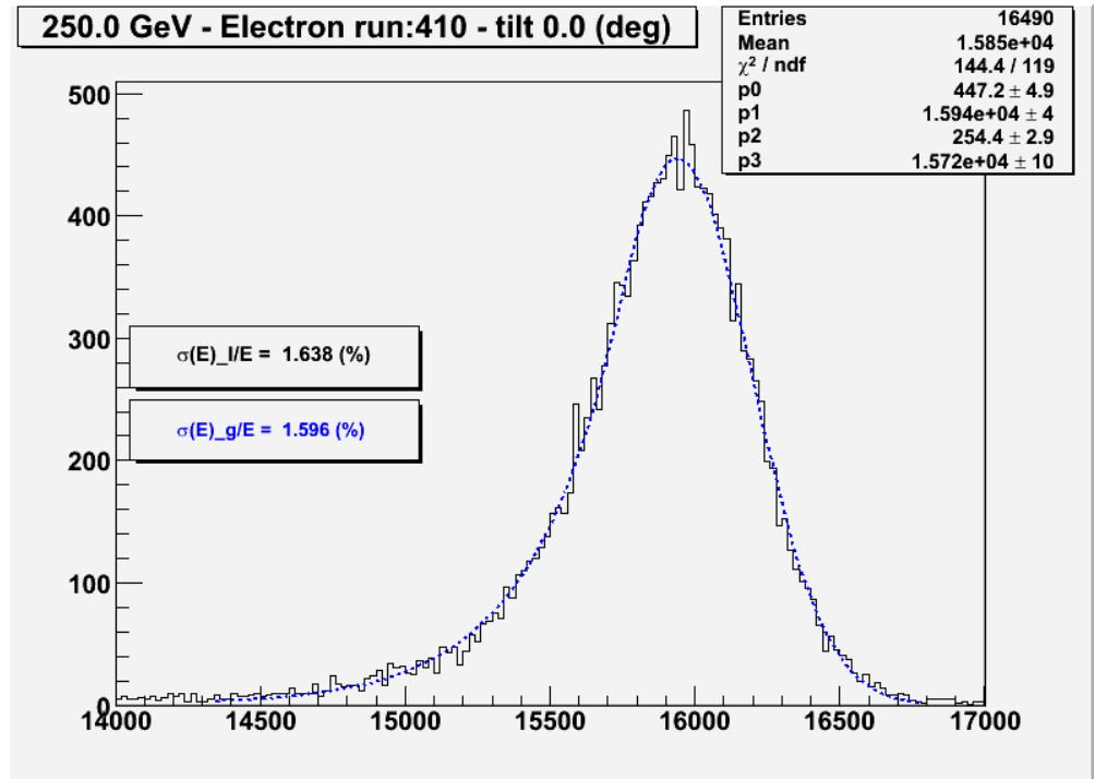
A better description of the energy distribution is given by a “Cristal Ball Function” (Gaussian + Exponential)
