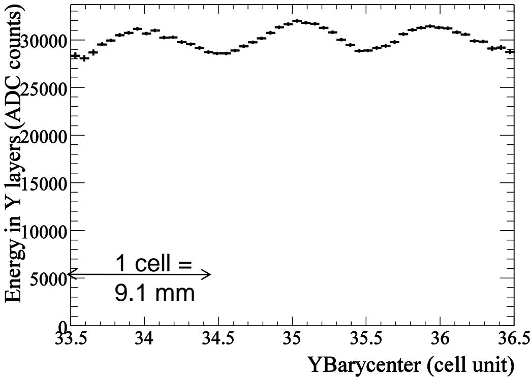
The energy measurement is sensitive to the impact point given here by the barycenter
