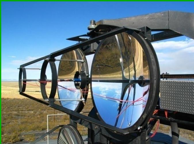
LIDAR at each fluorescence eye for atmospheric profiling - "shooting the shower"
