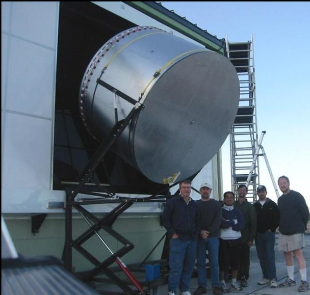
Drum for uniform illumination of each fluorescence camera
