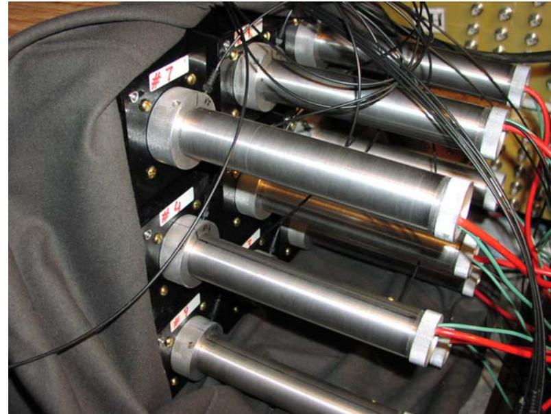
3x3 matrix of shashlyk modules and PMT attached to the modules
