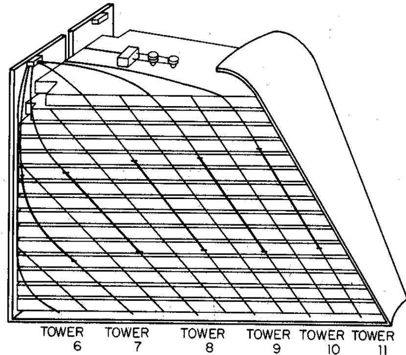
Fig. 2. Endwall calorimeter module. Module side faces are equipped with steel tubes positioned on the center lines of the towers and used for insertion of linear  $\gamma$  sources (section 4.2). The movable point source (section 4.3) is also schematically drawn: the source, moving inside a steel tube, traverses all the towers at a fixed longitudinal depth along scintillator center-lines.
