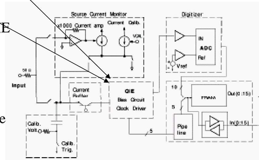
Fig. Simplified schematic of frontend (CAFÉ) card containing QIE and FADC
