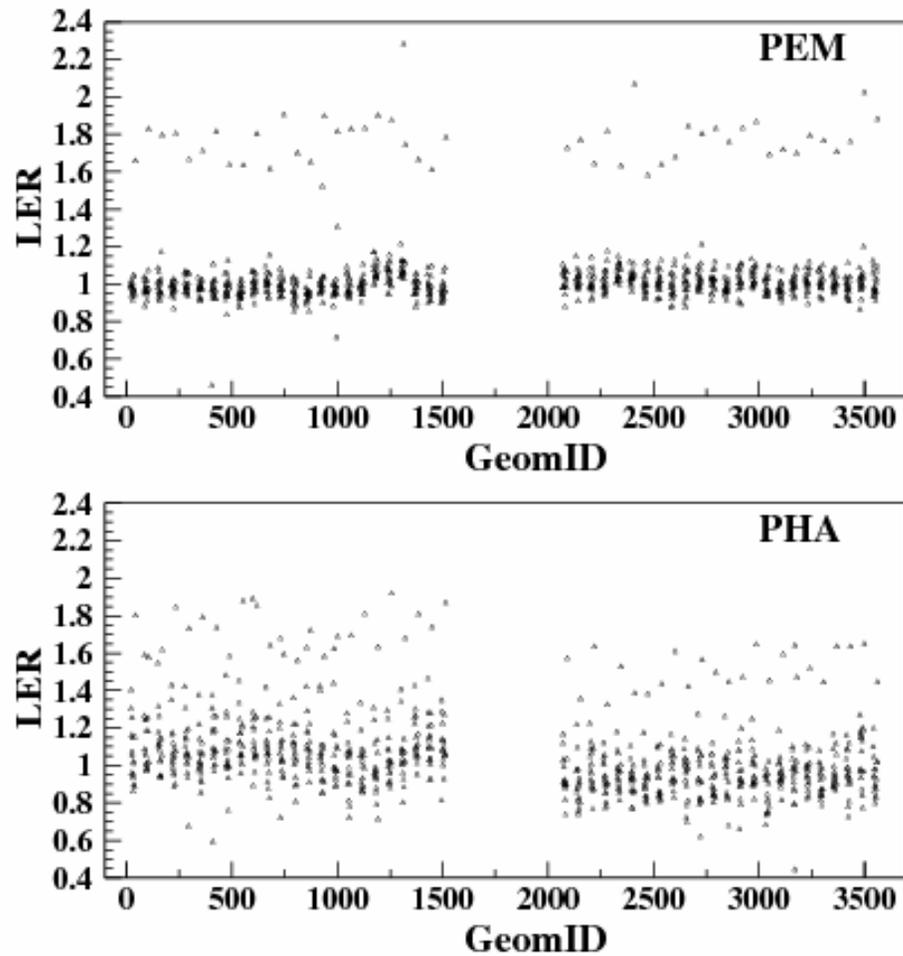
Figure 4: The Nov 2001 LERs for the PEM and PHA versus the geometrical ID. The west side of the detector are the points on the left side. Each vertical band corresponds to the towers in a wedge.
