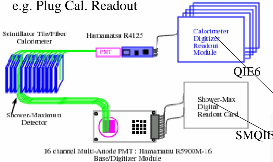
Need more (x2) dynamic range for run II so new f.e. readout electronics based on QIE (Q-integrator and encoder): custom-built 8-range ( $I/2 - I/256$ ) current splitter / integrator / encoder. Mounted on f.e. (CAFÉ) card together 10-bit FADC, Q-injection circuit and FRAM
