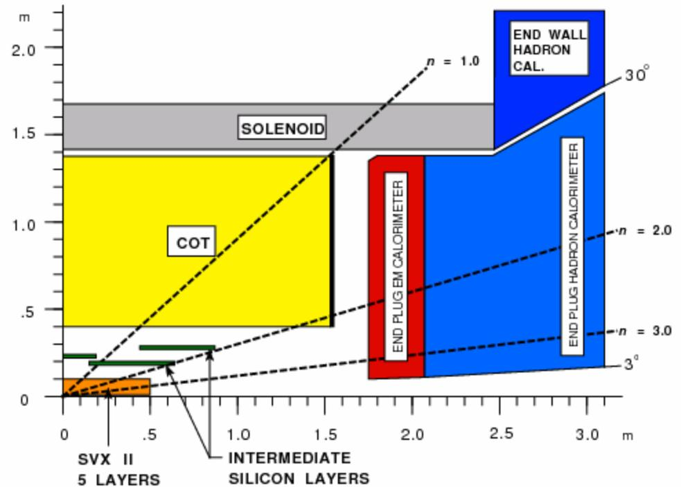
Figure 1.3: Longitudinal View of the CDF II Tracking System
