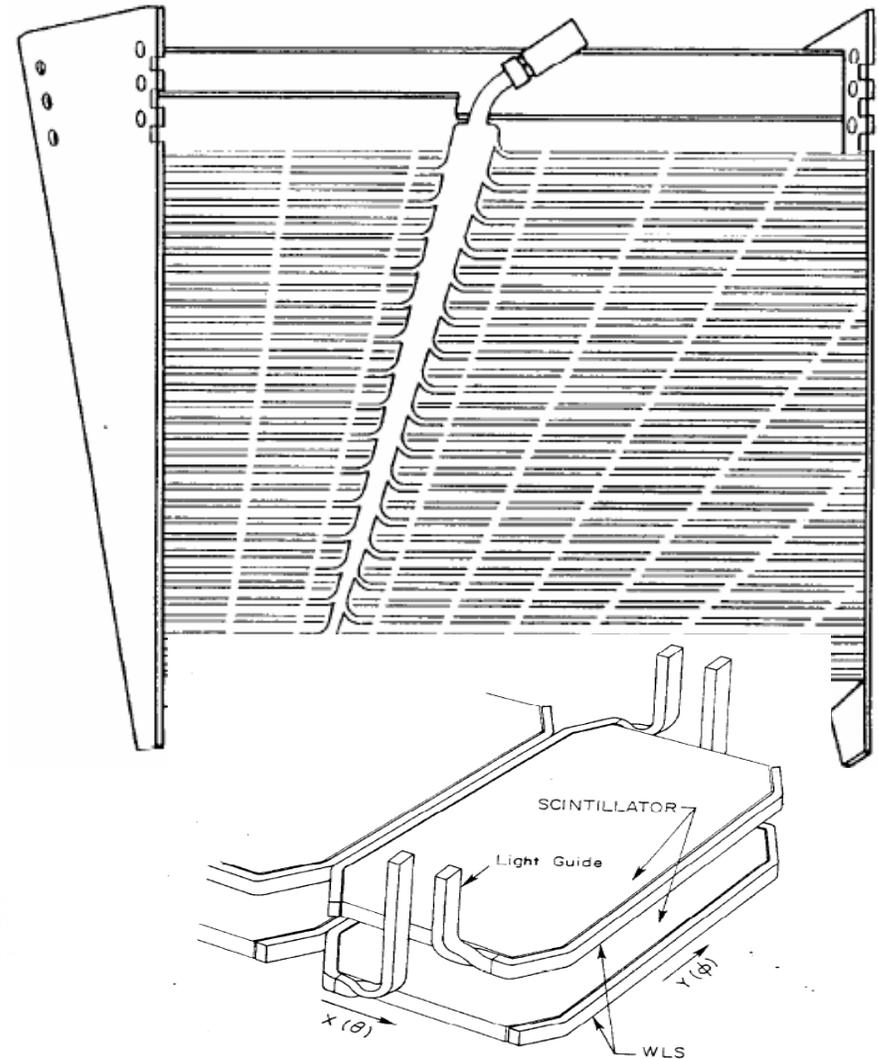
Fig. 4. Two WLS strips collect light from each scintillator layer. In the air gap between WLS and light guide, filters are inserted to ensure light output equalization for different layers of the same tower.
