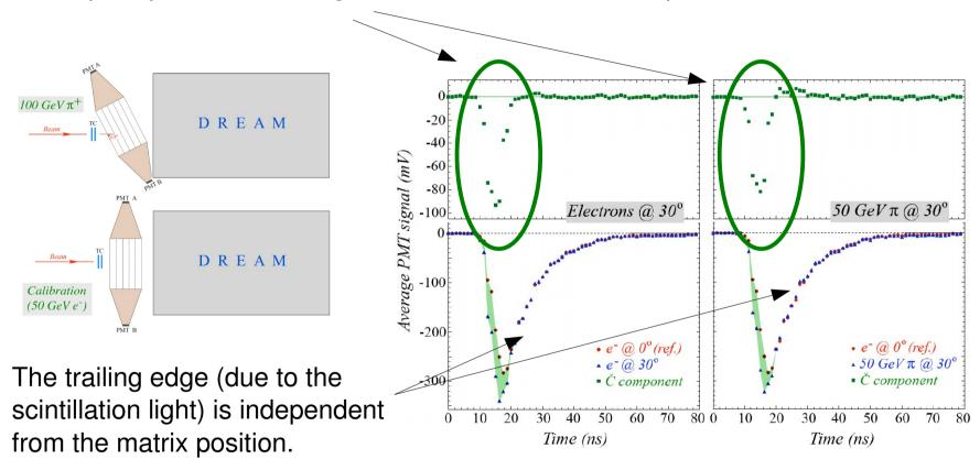
$\star$  With the tilted ECAL, the light-asymmetry (B-A)/(B+A) gives a measurement of the Cherenkov light ratio to the total signal which is a measurement of f;
