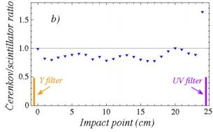
When the em shower has its maximum on the filter/window a large amount of Cherenkov light (but no scintillation light) is produced.
