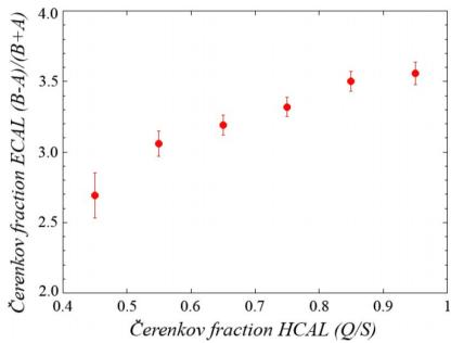
x A PWO-based ECAL is able to give precious information on the em content of the shower and to allow to correct the HCAL response.
