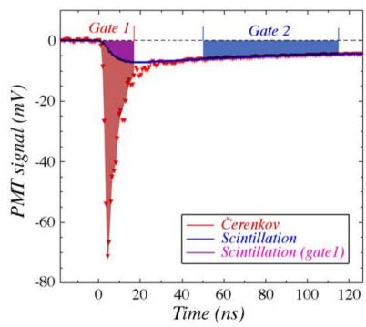
Once corrected for this effect Q1 and Q2 were calibrated to have C and S with distributions centred around 38 GeV in the run with 50 GeV electron beam (because of the lateral leakages).
