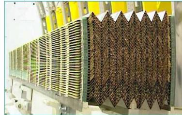
calorimeter module in cryostat (testbeam)
