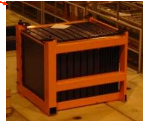
Scint. Strips-Fe Tail Catcher & Muon Tracker 5x100cm 2 strips ~5 λ in 16 layer
