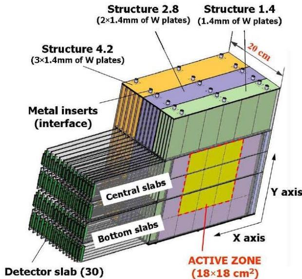
30 layers with variable sampling ratio (24 X0)
