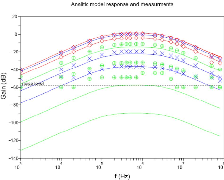
Figure 15: Model response and measurements made on hardware model
