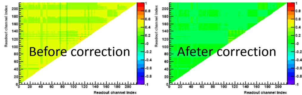
In test beam, **noise correlation** between channels is  $0.4207 \pm 0.0004$  MIP (mean),  $0.0551 \pm 0.0002$  (stdev) before pedestal shift correction and  $-0.0017 \pm 0.0003$  (mean),  $0.0519 \pm 0.0002$  (stdev) after **offline correction**
