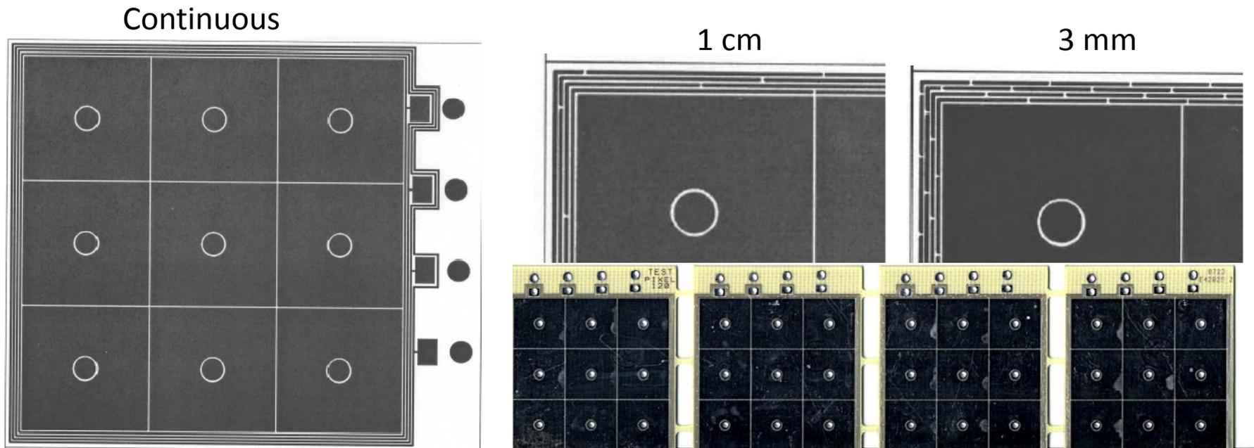
Figure 6: Copper epoxy made wafer model featuring 3x3 pixels and 4 continuous guardrings.
