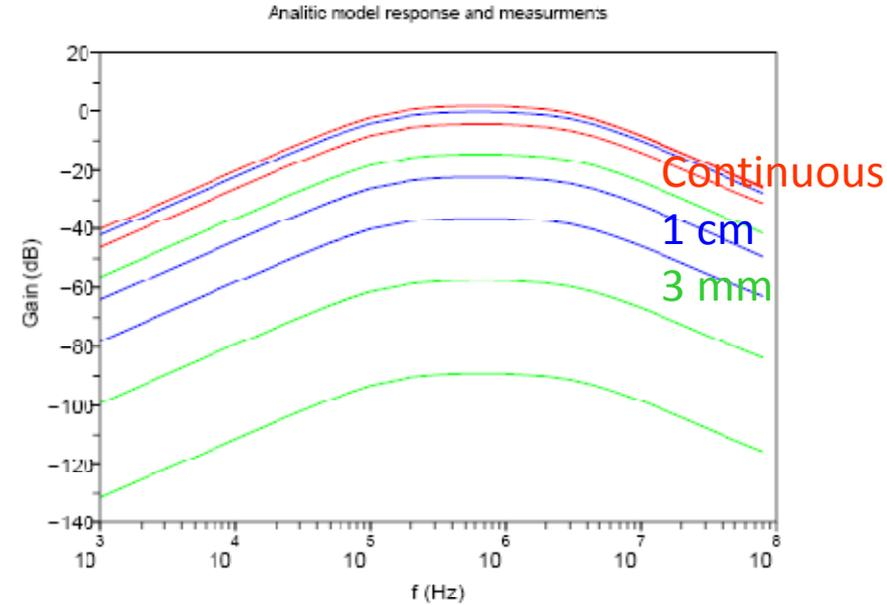
Figure 11: Model response (set for copper-epoxy model)
