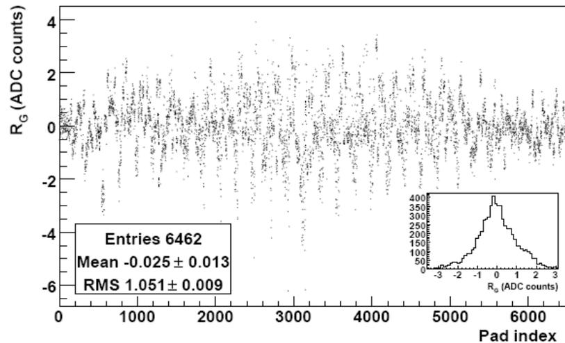
Pedestal can be corrected on an event by event basis to avoid pedestal shift
