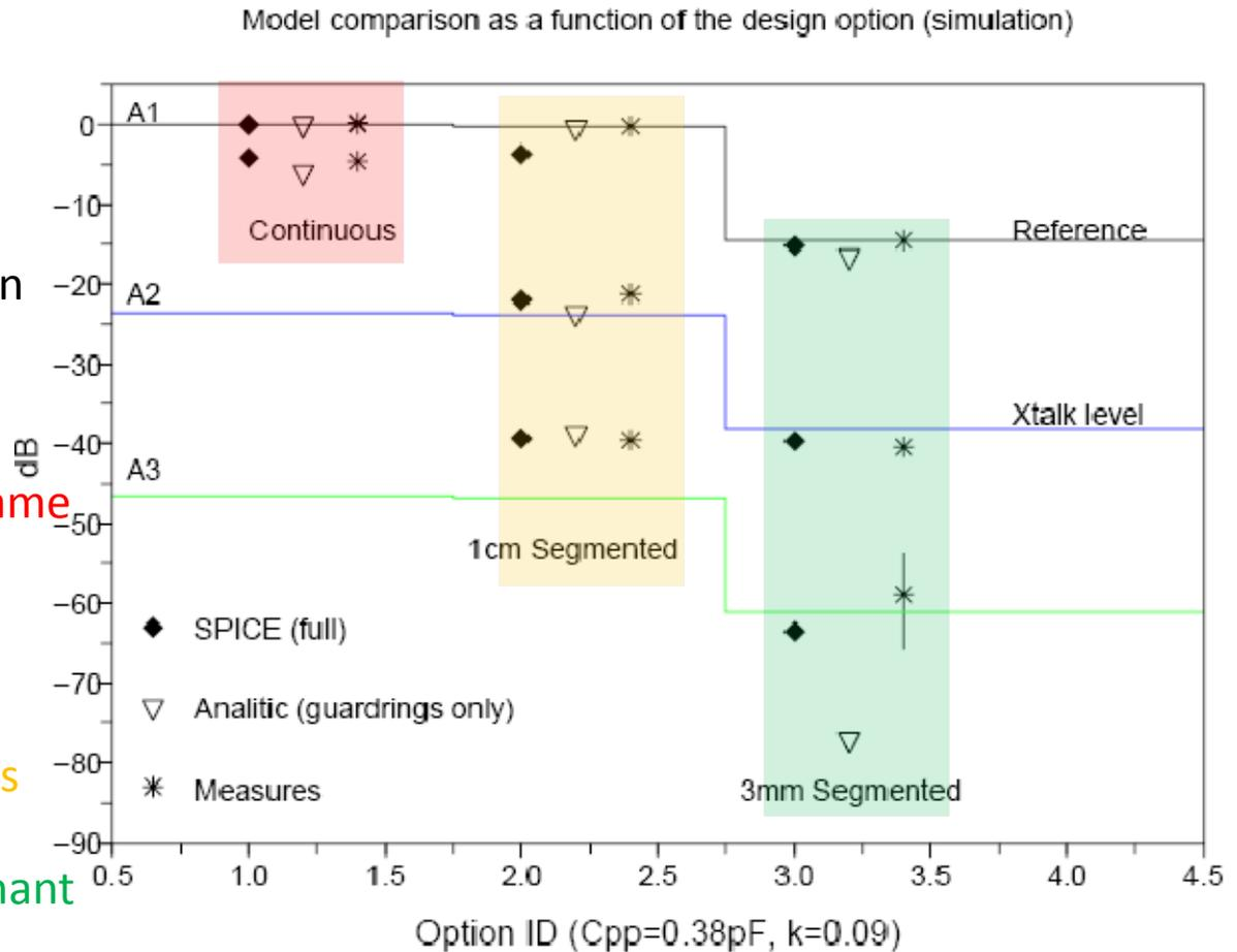
Segmented topology should limit square events effects to the pixel to pixel crosstalk
