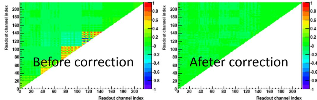
Coherent Noise (baseline shift) **induced by signal** was measured and can be corrected in the data.
