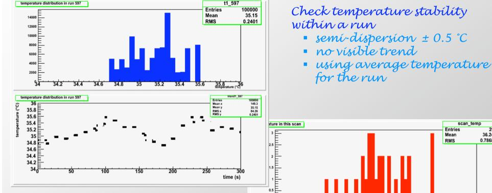
Check temperature stability within an angular scan performed at the same nominal temperature
