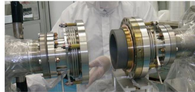
HOM beamline absorber installed on the cavity string inside the clean room (courtesy to Cornell).
