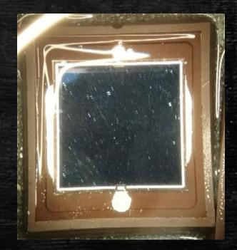
DC 184 has been tested on new PDs with 6 hours waiting time and ~300 um spacer.
