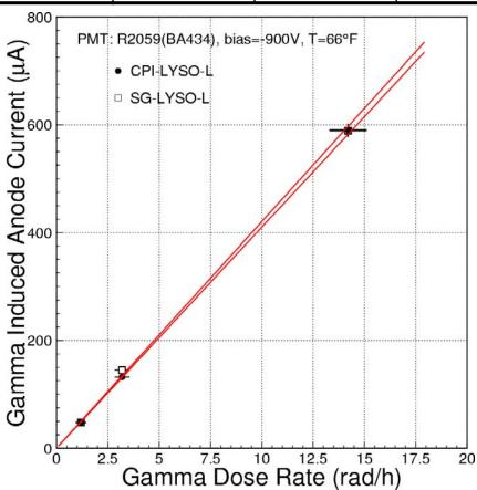
$\gamma$ -ray induced PMT anode current can be converted to the photoelectron numbers (Q) integrated in 100 ns gate. Its statistical fluctuation contributes to the readout noise ( $\sigma$ ).
