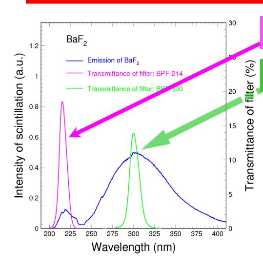
Transmittance for filter BPF-214 (fast component)
