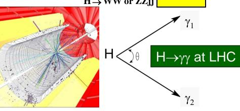
σm / m = 0.5 [σE<sub>1</sub>/E<sub>1</sub> ⊕ σE<sub>2</sub>/E<sub>2</sub> ⊕ σθ /tan(θ/2)], where σE / E = a / $\sqrt{$  E ⊕ b ⊕ c/E and E in GeV
