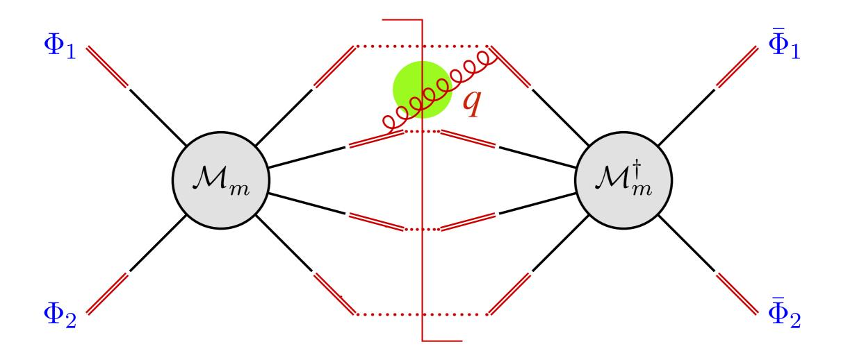
$\mathscr{W}_m$  at NLO is obtained by computing soft Wilson line matrix element or, equivalently, from product of soft currents  $J^a_\mu(q)$ .
