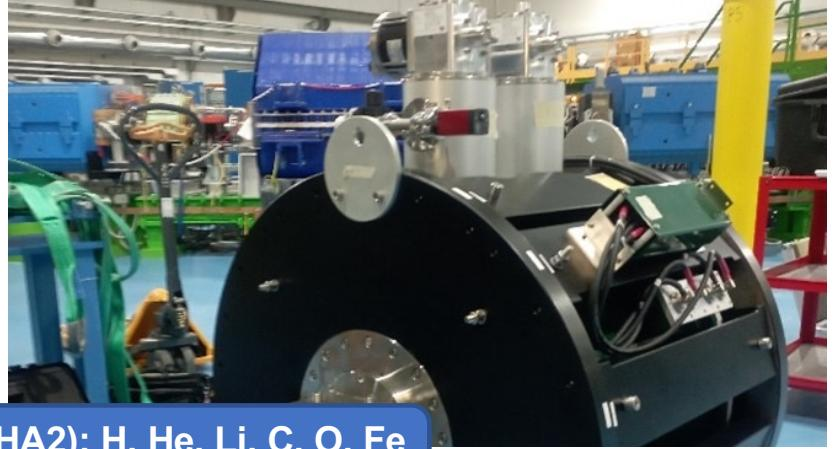
New superconducting ion source (AIsha2): H, He, Li, C, O, Fe
