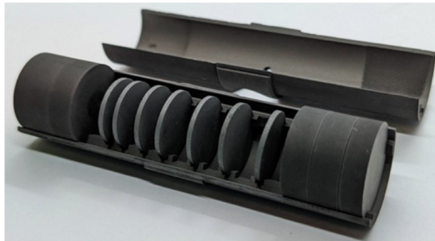
The target represents the heart of SPES in which the proton beam is converted in radioactive ions by means of nuclear reactions, for nuclear physics studies or medical isotopes research
