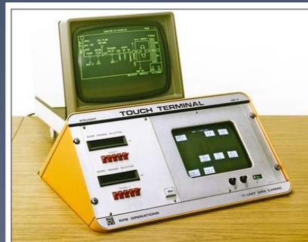
The Touch Terminal as developed for the Antiproton Accumulator (AA).
