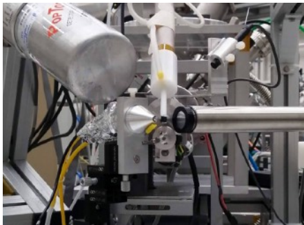
External beam for low-current non-destructive PIXE, PIGE and RBS/EBS analysis of cultural heritage
