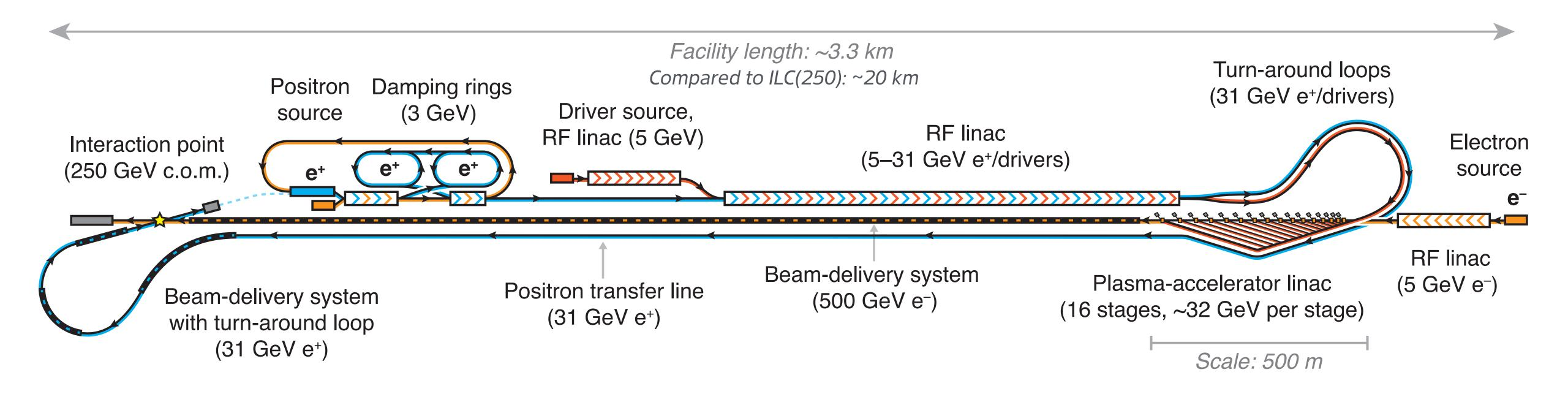
Length =  $\sim$ 3.3 km: similar to XFEL@DESY  $Cost = ~2.1 B \in +/- 25\% = ~ILC/4 = ~EIC$
