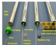
Straw tube components (for PANDA-STT [1])
