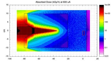
FLUKA simulation of the absorbed dose in a sample of LaBr and surrounding area at the irradiation point
