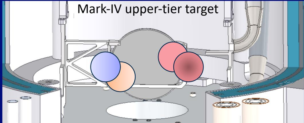
In the case of MARK-IV, due to its design, the accurate position of FOV matters due to part of FOV on water, another part on W target having harder nFlux
