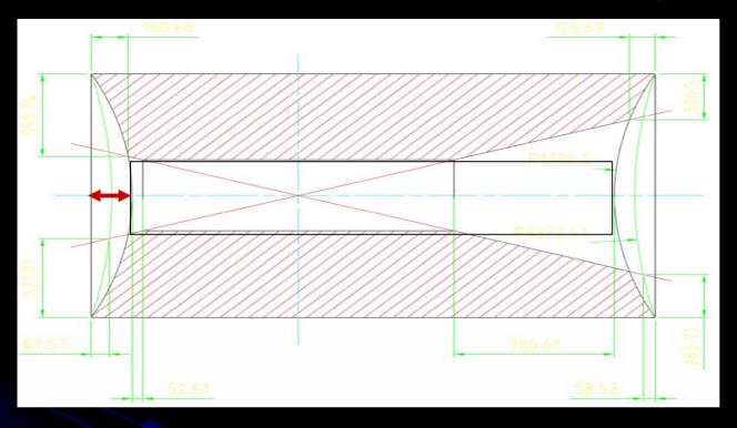
Thickness O(4mm), or  $0.015 X_0$ sagitta=200mm  $\rightarrow d_{max200} \le 0.5$ mm sagitta=100mm  $\rightarrow d_{max100} \sim 2xd_{max200}$
