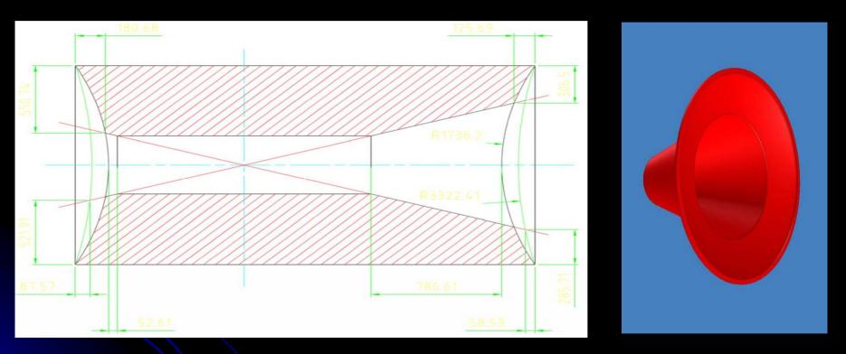
Thickness O(4mm), or  $1.5\% X_0$  (perp. to walls)  $d_{max}\sim 0.5mm$
