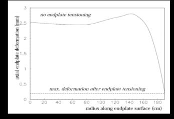
Total load due to tension of 27k wires in BABAR DCH is ~3.5 tons
