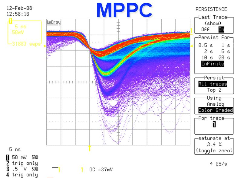
**Pulse height spectrum when using charge amplifier (S10362-11-025U,  $M=2.75 \times 10^5$ )**
