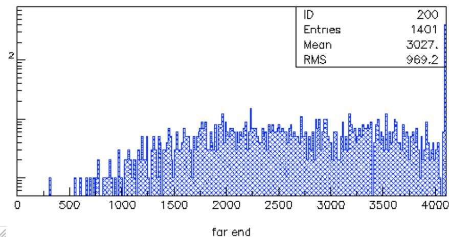
ADC spectra for a kuraray T11-300 fiber about 4 m long in a surface groove
