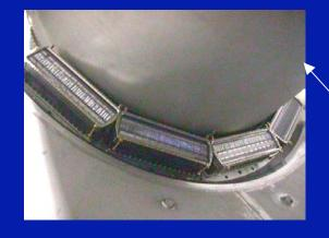
Inner SOB cylinder has to be removed
