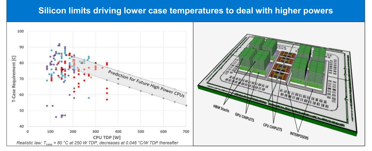
Stacked structures increase thermal resistance and force package temperatures lower
