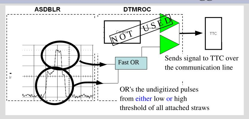
Pulse at TTC board: "OR" of ~240 attached straws
