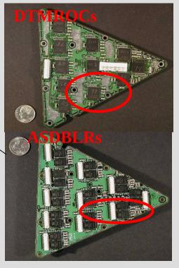
"DTMROC": "Drift Time Measurement Readout Chip"
