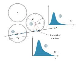
• Measured ToT correlated with the sum of the energy depositions of primary ionization electrons
