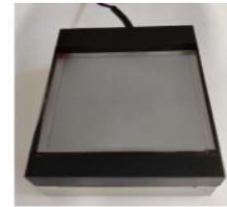
MCP with 64 x 64 anode pads (Photek)
