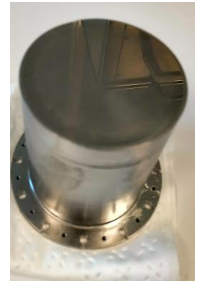
QPR sample after second polishing step
