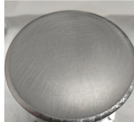
QPR sample after first polishing step
