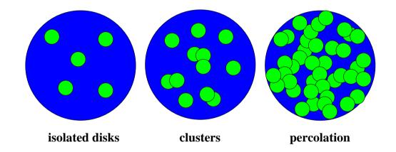
• 3-d: N spheres of volume  $V_h$  in box of volume V, with overlap increase density n=N/V until largest cluster spans volume: percolation
