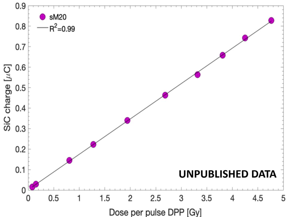
OPEN-FIELD NO APPLICATOR 3 mm<sup>2</sup> SiC detector
